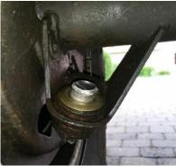
\*\*NOTE – Terrafirma TF169 +5" shocks have pin top mounts instead of the conventional ring, this is to allow unrestricted articulation and movement of the mounting point. To allow these shocks to be fitted it is necessary to also fit TF519 extreme long travel rear top shock mounts that are simply bolted to the original mounting points. These are sold separately and not included with the shock absorbers.
