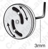
Refer to diagram. The adjustable drive key adaptor locking screw is accessed from the rear 3/8" drive socket Loosen the screw with a 3mm hex key and then adjust the pins to fit the corresponding holes or sockets in the caliber piston.
